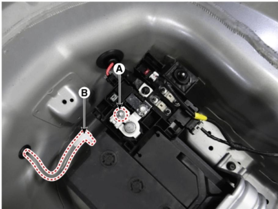
7. Remove the mounting band (A).
